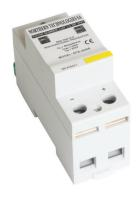
The NTS-24/48 provide economical and reliable protection to primary panel boards and power distribution systems. Internal thermal disconnect devices ensure safe isolation during sustained and abnormal events on the distribution network, or at end of life. Visual indication and voltage free contacts is provided for remote signaling if replacement is due.
